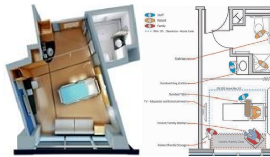
Figure14: The furniture layout of patient room to afford a wide variety of functions such as contacting other patient/treatment staff /family zone.
